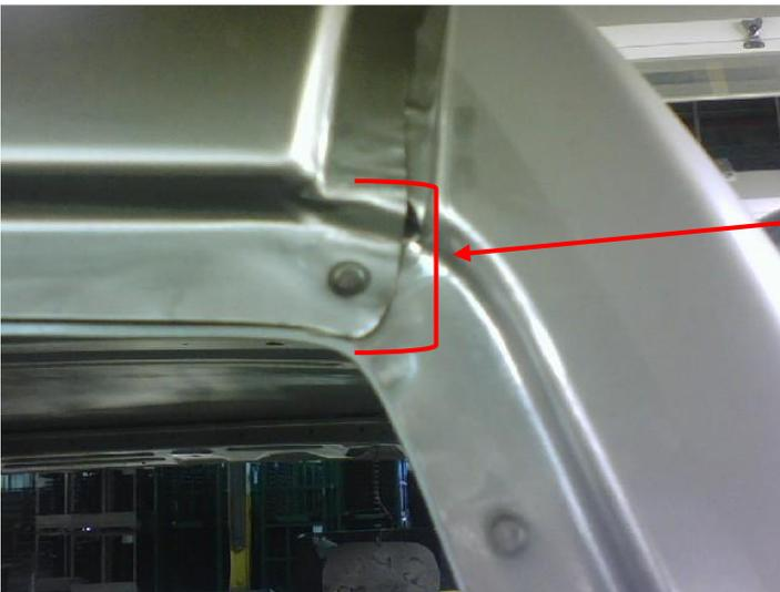
Apply clear sealer on entire length of seam indicated within the bracket
